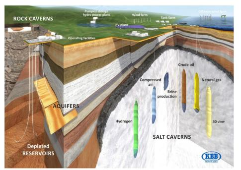
1 salt cavern can contain 6,000 ton hydrogen Equivalent of 17 million Tesla Power walls
