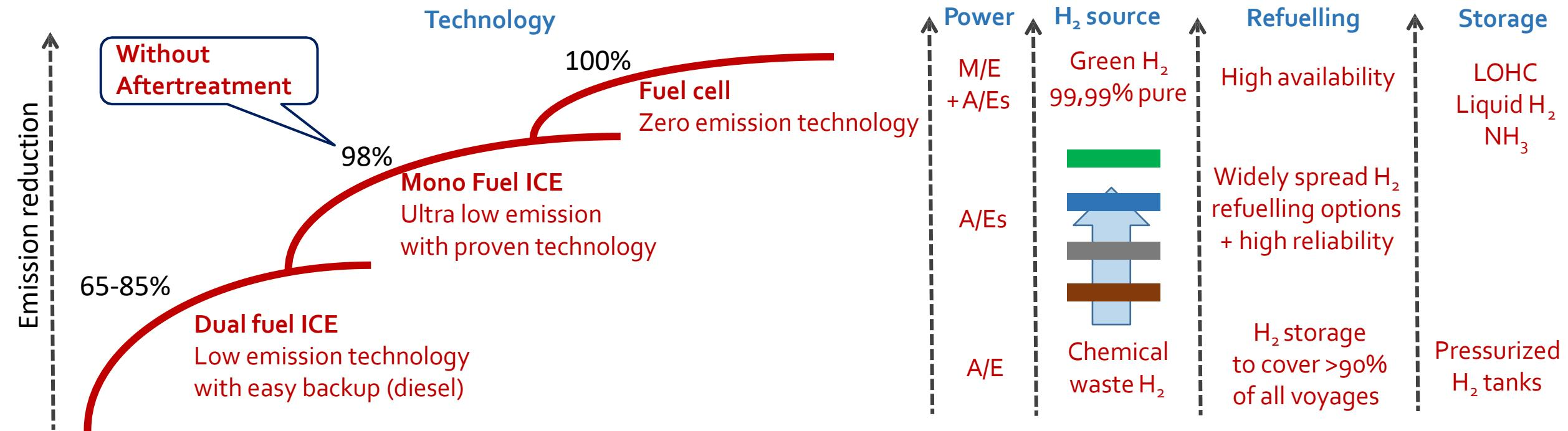
→ Dual fuel technology is a first step towards the zero emission goal, while the service can be guaranteed as one always can rely on diesel
