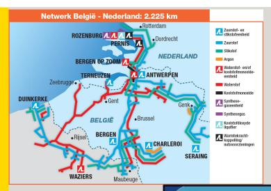
Pipeline network of Air Liquide & Air Products, hydrogen in RED
