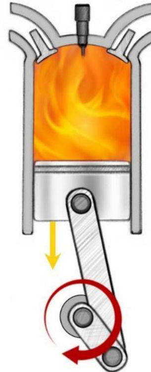
Diesel auto-ignites (due to high temperature and pressure) and co-combusts with all the H_2 , forcing the piston down during the power stroke
