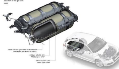
Audi A3 Sportback g-tron Fuel and Gasoline Structure of the gas tank 06/12
