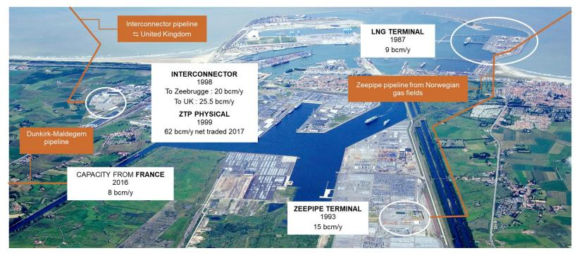
Zeebrugge area : throughput capacity of ~ 57 bcm/y = over 12% of border capacity needed to supply Europe
