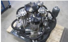
Compression (ionic compressor)
