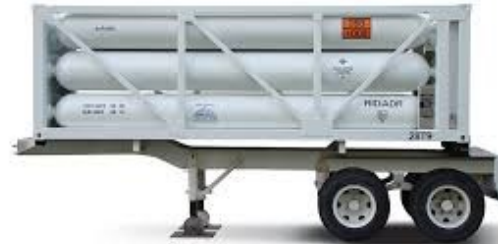
Tube Trailer 30 Mpa ~ 300 kg
